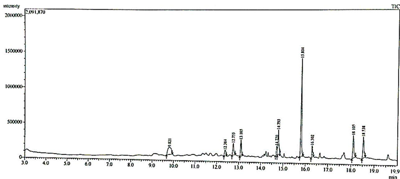
Figure 3. GC-MS chromatogram of EF1
