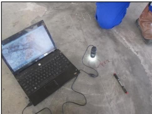
**Gambar. 5** Alat ukur field microscope crack
